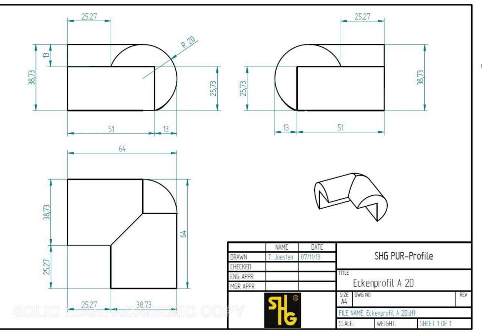
Technical Data Sheet Protective corner, two-dimensional Type A (2D)
